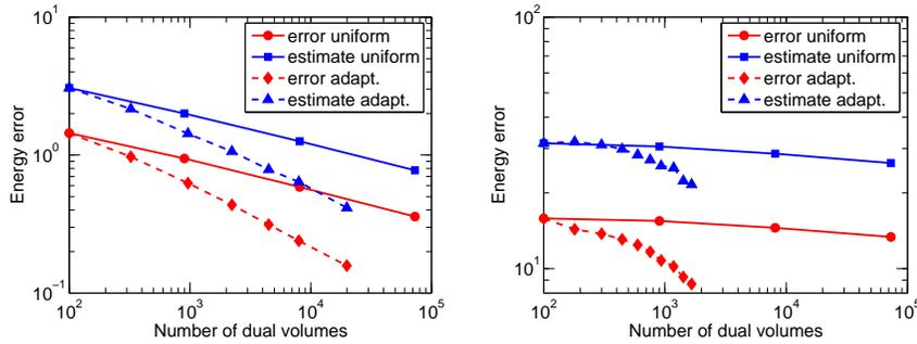
Figure 5: Estimated and actual energy error against the number of dual volumes for case 1 (left) and case 2 (right), potential-based postprocessing and estimates
