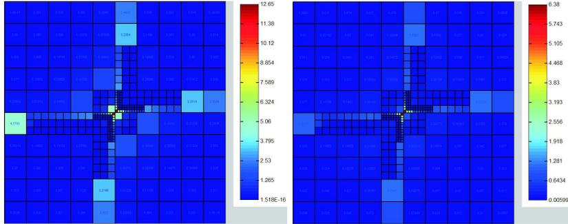
Figure 4: Estimated (left) and actual (right) error distribution, case 2, potential-based postprocessing and estimates
