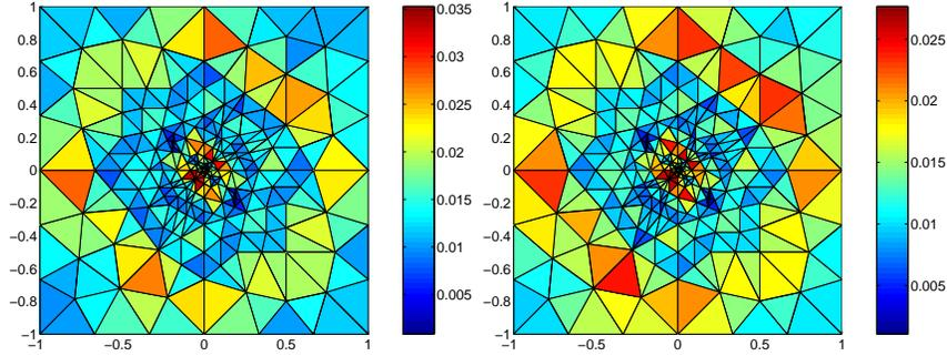
Figure 2: Estimated (left) and actual (right) error distribution, case 1, flux-based post-processing and estimates
