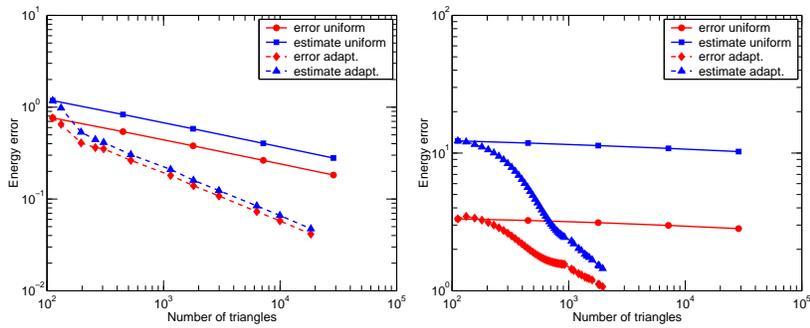
Figure 3: Estimated and actual energy error against the number of elements for case 1 (left) and case 2 (right), flux-based postprocessing and estimates
