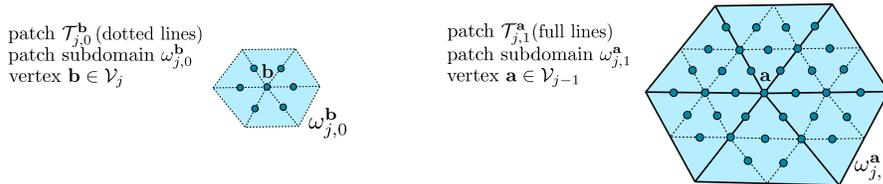
FIG. 2. Illustration of degrees of freedom ( $p' = p = 2$ ) for the space  $V_{j,0}^{\mathbf{b}}$  associated to the “small” patch  $\mathcal{T}_{j,0}^{\mathbf{b}}$  (left) and for the space  $V_{j,1}^{\mathbf{a}}$  associated to the “large” patch  $\mathcal{T}_{j,1}^{\mathbf{a}}$  (right). The mesh  $\mathcal{T}_{j-1}$  and its refinement  $\mathcal{T}_j$  are defined in bold and dotted lines, respectively.
