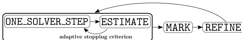
Scheme 2: Paradigm of an inexact hp -adaptive algorithm comprising an inner (algebraic) loop and an outer ( hp ) loop; both loops are driven adaptively.
