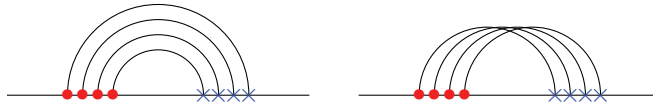
FIG. 1.1. On the left: optimal plan associated with a concave cost. On the right: optimal plan associated with a convex cost. Supplies are represented by circles and demands by crosses.
