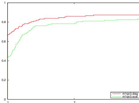
Fig. 2. Performance profiles of the diagonal (`m1qn3.diag`, red top curve) and scalar (`m1qn3.scal`, green bottom curve) running modes of `M1qn3` on 143 unconstrained problems of the CUTER collection, comparing the number of function evaluations; relative performance (abscissa) in  $\log_2$  scale
