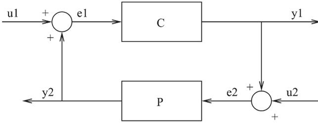
Fig. 1 Closed-loop system
