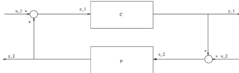
Figure 1. Closed-loop system.
